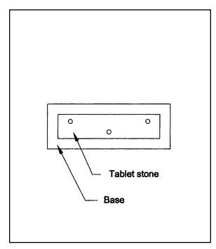
When using dowels in the repair it is best to offset the middle dowel to avoid the chance of weakening the marker along a bedding plane.
