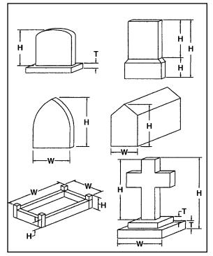
Full and accurate measurements are necessary information. Standardized criteria must be consistently used throughout the process. In this illustration several types of stones and the points of measurement are identified.
