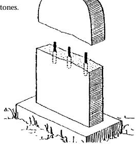
Repair of snapped marker using nylon or stainless steel dowels epoxied into their holes. Dabs of epoxy can be used to secure the two pieces together while grout can be injected after the epoxy has cured to reinforce the repair. Knife grade epoxy can be used for the dabs of adhesive and for securing the dowels to the holes.
