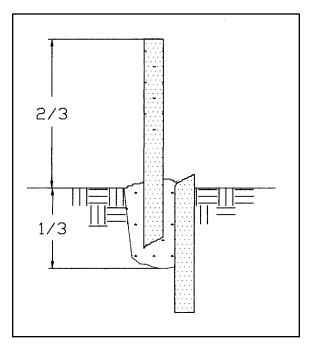
As a temporary fix simply resetting the broken piece in front of the parent stone is a reasonable action and one that can quickly improve the look of the cemetery.
