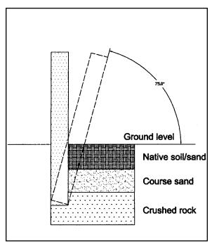
Straightening a marker is a common task done usually when the marker is out of plumb by 15 or more degrees. Always use caution when moving a stone. Trying to force a stone can cause it to snap.
