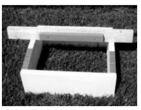
A die is made from lumber so that when inserted into the uncured cement, a slot will be formed and the tablet stone can be inserted when the cement has cured.
