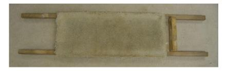
Before moving the broken headstone and parts, ensure it is structurally supported to prevent any new damage. I use a wooden platform that allows the headstone to lie on a carpet pad. The stone is loosely strapped to the platform and two people can lift and move the headstone without damage.
