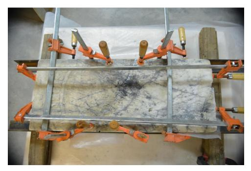
It must be clamped properly to allow it to be turned on its' side, as in the picture above. You may have to epoxy some pieces together on a flat table before you use a raised platform. Case in point...The lower left bottom of the pictured headstone. The small piece was epoxied on the flat table.
