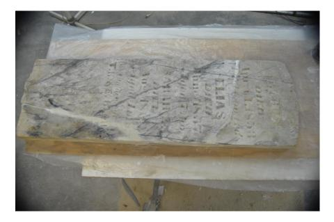
Headstone epoxied with rough infill. Infill was smoothed out before the mixture cured and after about two weeks, the stone was returned to the cemetery.
