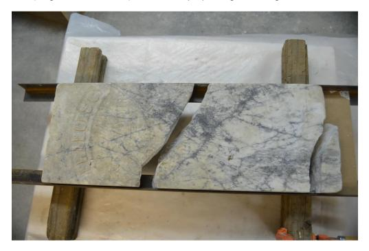
A benefit of a raised platform is that it allows for the clamping of the outside edges of the headstone to the angle braces.
